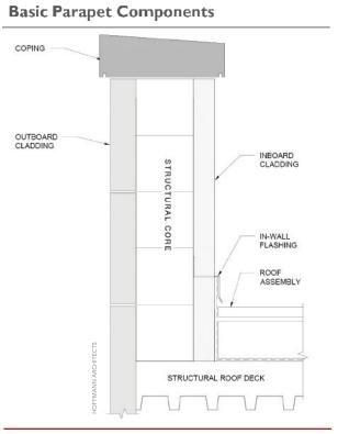
materials and building systems, modern parapets, constructed of diverse materials from reinforced concrete to masonry to steel, have since incorporated provisions for structural reinforcement, along with accommodations for moisture mitigation, such as in-wall flashings and vapor barriers.
