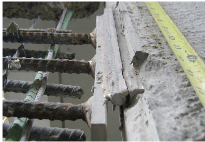
▲ Connection fracture from high slug position.
