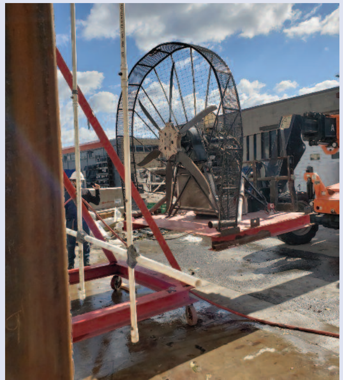
Fans simulating high winds are used for dynamic water testing.
