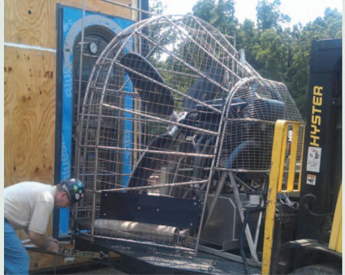
*In the lab: Wind and water test preparation for a window PMU.*
