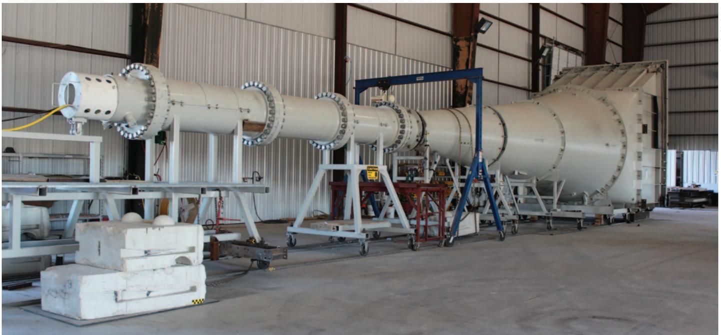
*Shock-tube apparatus for blast-resistance window testing.*
