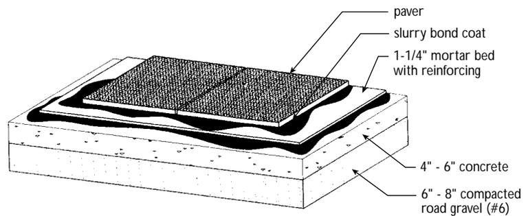
Illustration C: Solid-set paver or closed-joint system.
