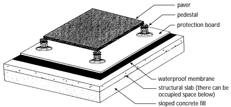
Illustration A: Paver-on-pedestal or open-joint system.
