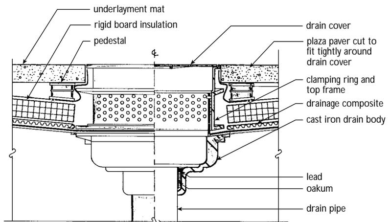
Illustration B: Plaza drain detail for open-joint system.
