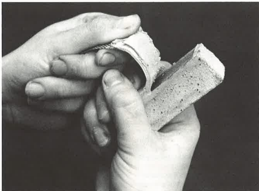
testing materials beforehand will show whether proper adhesion is attained
