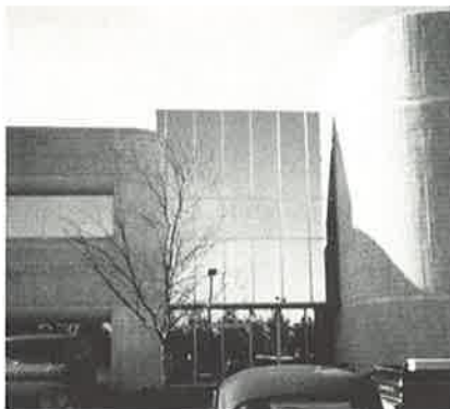
reflective glass cuts down solar gain
