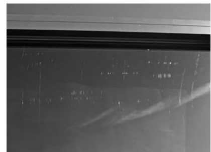
A Scratches and hairline cracks.
