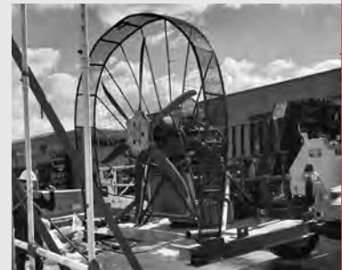
▲ Fans simulating high winds are used for dynamic water testing.
