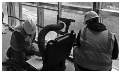
Window performance testing establishes thermal efficiency and moisture protection.
