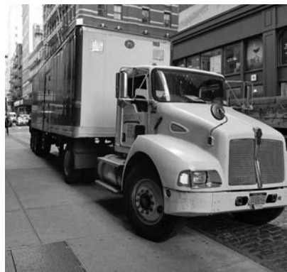
▲ Delivery trucks on sidewalks may add weight beyond what historic vaults can bear.
