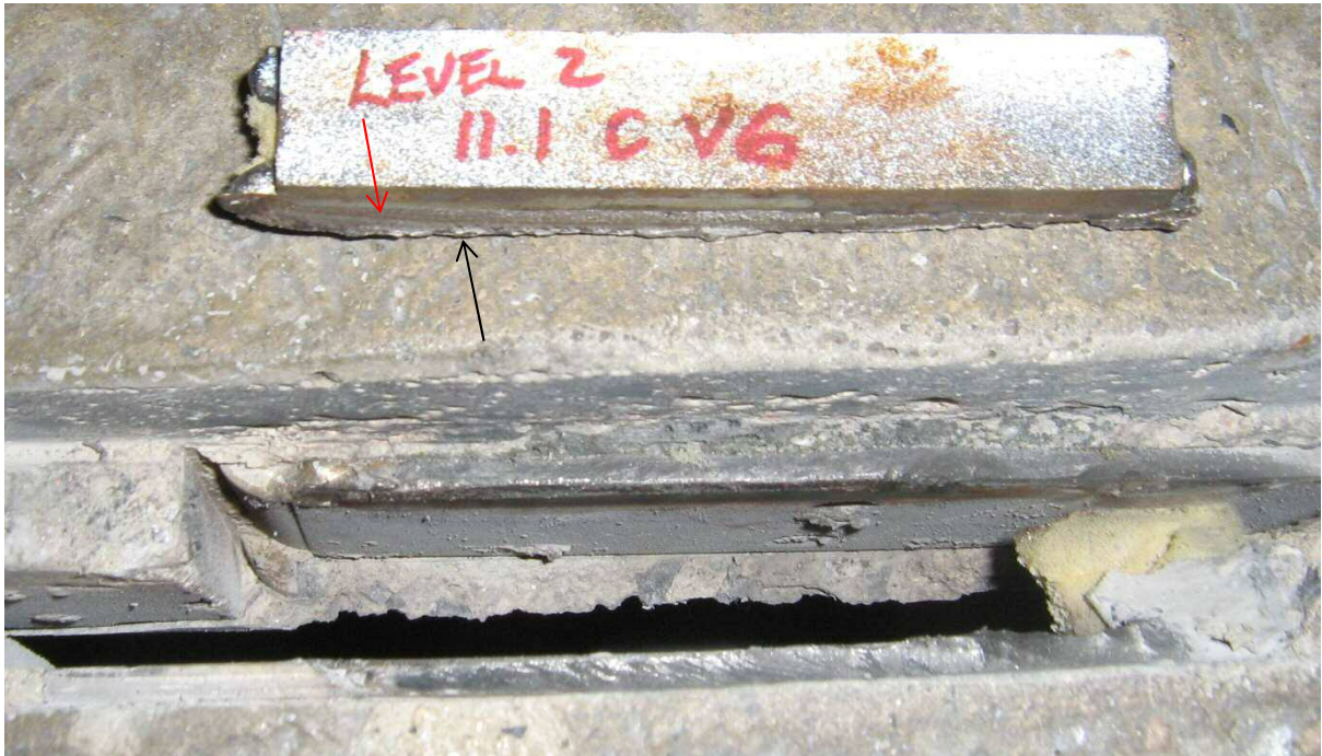
Figure 9 Fatigue fracture at flat erection bar (shown upside-down). Note uniform and burnished crack propagation zone and linear striations at face of weld fracture (red arrow) and abrupt fracture at face of weld (black arrow).
