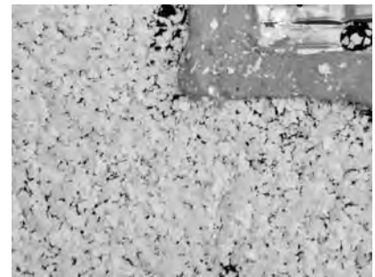
▲ Reflective granules on a high-albedo cap sheet direct solar heat away from the roof.
