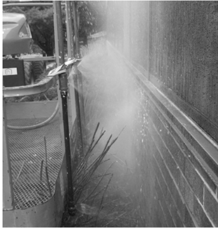
▲ A leak investigation in process: water is applied to the exterior envelope at the specified test pressure, whereupon the design professional documents water penetration at the interior.
