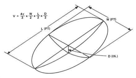
Nomograph assumes ponded water on a sagging roof will take the approximate shape of an ellipsoid, the volume of which is equal to the product of its semiaxes multiplied by 4 pi/3.
