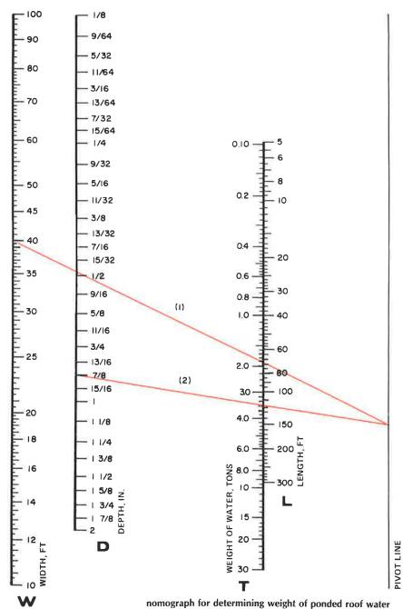
**Solution:** Align 40 on scale *W* with 70 on scale *L* and extend to pivot
