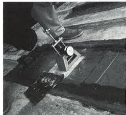
The substrate must be tested for pull-out resistance to determine the most appropriate fasteners.
