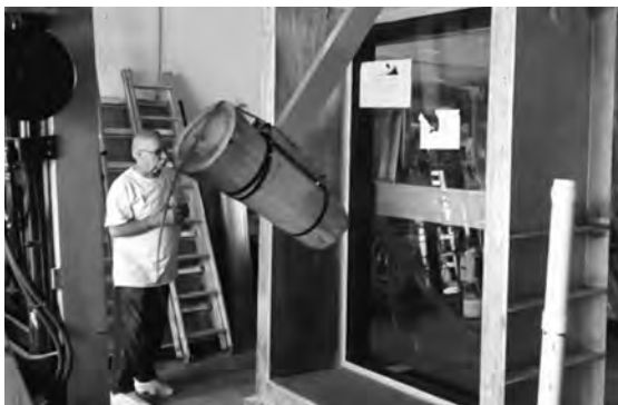
▲ Flood debris testing of a proposed window assembly.
