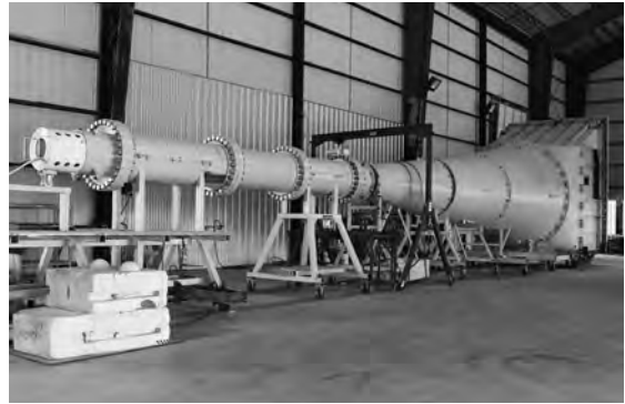
▲ Shock tube apparatus for blast resistance window testing.
