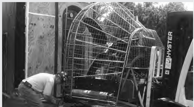
▲ In the lab: Wind and water test preparation for a window PMU.
