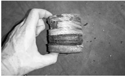
▲ Test cores may be used to evaluate conditions within a roof assembly.
