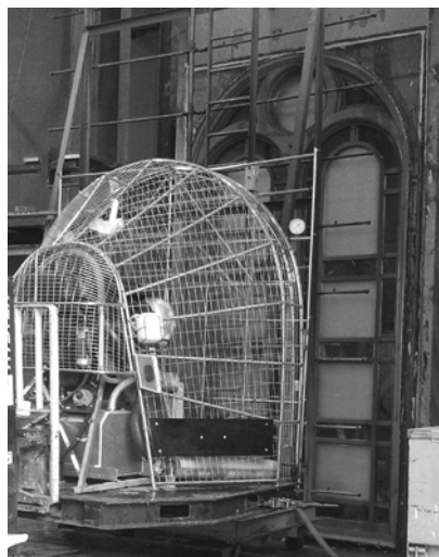
▲ High-powered fans or propellers are used to establish dynamic air pressure differences across a test sample.
