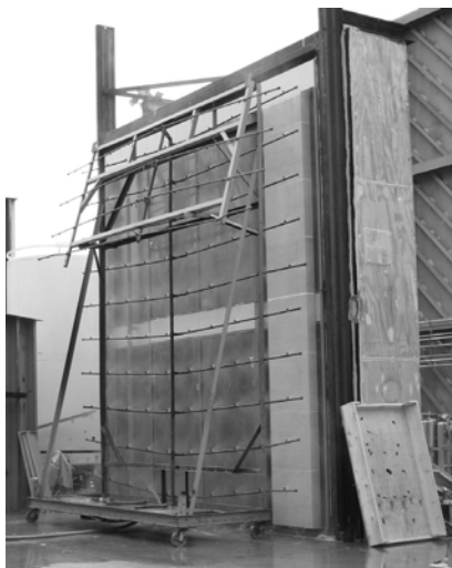
▲ Off-site spray rack testing allows the design professional to verify water-tightness of the proposed assembly.
