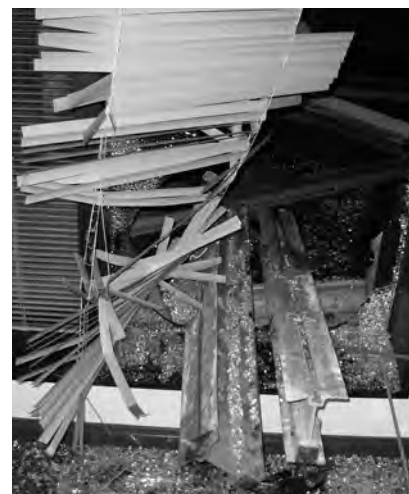
A In high winds, these steel beams became dangerous projectiles.
